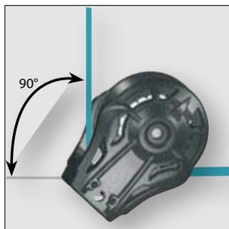
For a 90° angle: The load factor will be 140%. A load of 100 Kg on the line will represent a load of 140 Kg on the block.
